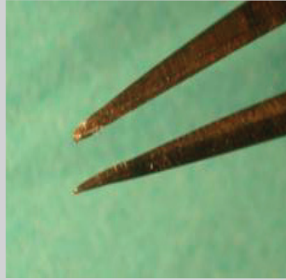
Straighten the points as much as possible with a pair of needle nosed pliers. Extremely bent bits will probably break off when straightened.
