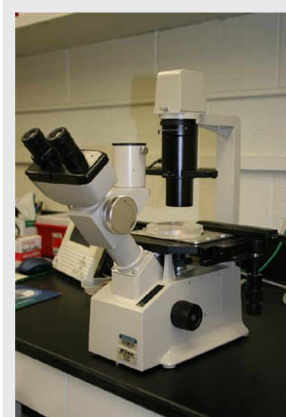
Figure 1. An inverted microscope has a light source above the stage while the objectives are mounted on a nosepiece below the stag. (Photo Jan Byrne, Michigan State University)
