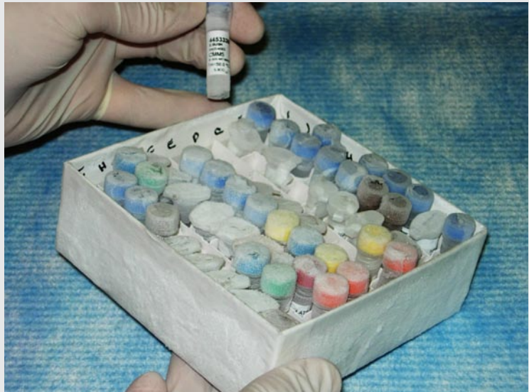
Figure 2. Fiberboard storage boxes with tube dividers can be numbered/lettered to correspond with primer/probe inventory entries in an Excel spreadsheet.
