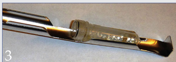
Fig. 1. 20L dewar for liquid nitrogen storage. Fig. 2. Plant tissue placed in 2.0 ml microcentrifuge tube with 2.5 mm glass beads. Fig. 3. Tube is clipped onto stick and ready for immersion in liquid nitrogen. Fig. 4. Four cryocanes are squeezed together to make one long stick.
