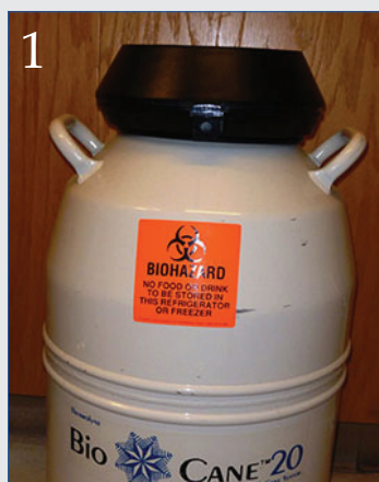
Fig. 1. 20L dewar for liquid nitrogen storage. Fig. 2. Plant tissue placed in 2.0 ml microcentrifuge tube with 2.5 mm glass beads. Fig. 3. Tube is clipped onto stick and ready for immersion in liquid nitrogen. Fig. 4. Four cryocanes are squeezed together to make one long stick.
