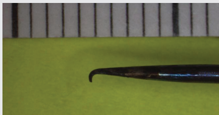
Fig. 1. A "modified" dissection needle useful for inoculating bacteria into pepper fruit. Small tick marks are millimeters.
