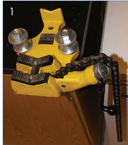
Fig 1. The bench chain vise is mounted on the right end of the counter. Mounting at the end of the counter is recommended since you turn a handle to tighten the chain. The composite material of lab benches is hard, so use a sharp drill bit and a drill with variable speed. We drilled slowly to prevent friction and damage to the counter.
