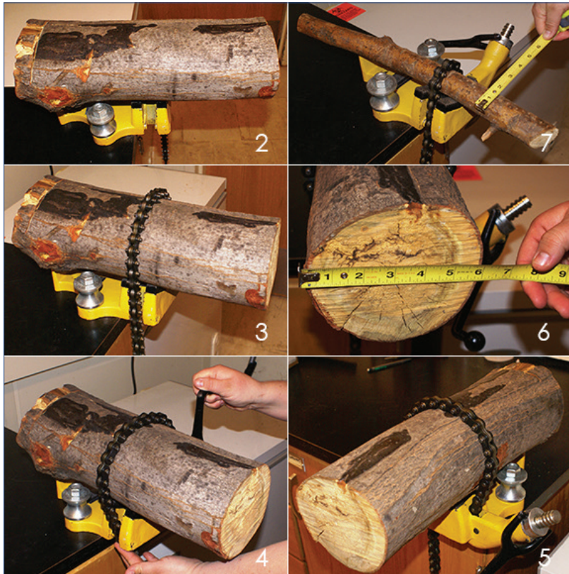
Fig 2. Lay the log or branch on the top of the vise. The portion that you desire to cut should point towards you, away from the counter.
