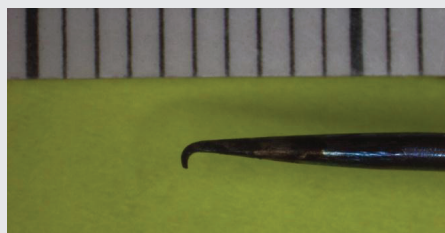
Fig. 1. A "modified" dissecting needle useful for inoculating bacteria into pepper fruit. Small tick marks are millimeters.
